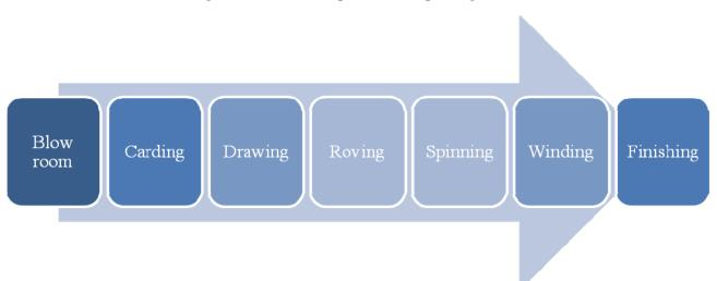
Figure 13: Production processes in spinning
